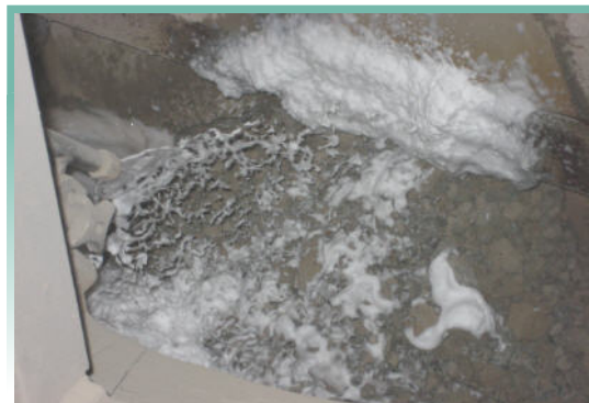
Foam spray added to limestone at a crusher inlet
